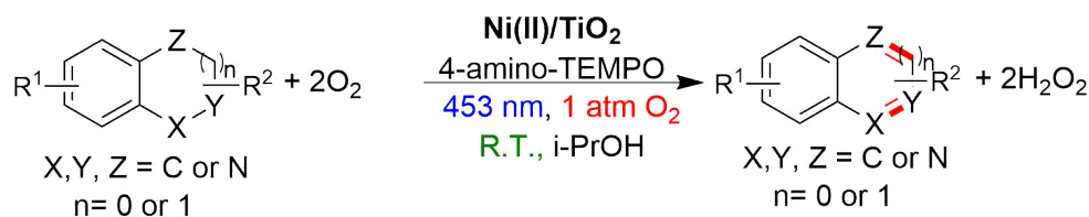
Scheme 4.1: Dehydrogenation reaction conditions of N-heterocycles in O 2 atmosphere.
