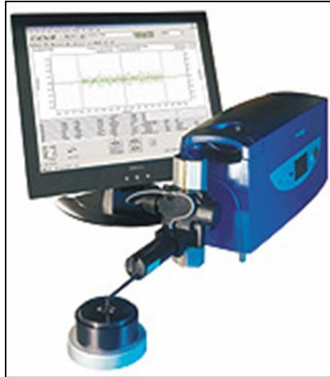
Figure 4.1: Experimental set-up of a profilometry measurement
