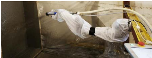
Figure 9: Experimental setup for concrete spraying with UR5 robot
