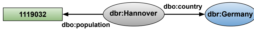
Figure 2.2: Concrete RDF Graph Instance from DBpedia [Aue+07] depicting a resource (the city of Hanover) and two relations about it. To which country it belongs (Germany) and its population (integer number).
