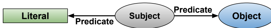
Figure 2.1: RDF Graph showing two RDF triples. Each triple consist of a subject (resource indicated in an oval shape), a predicate (of a verb, indicated as a directed arrow), and an object which could be a literal (simple values indicated via rectangles) or a resource (a dereferencable entity indicated via ovals).
