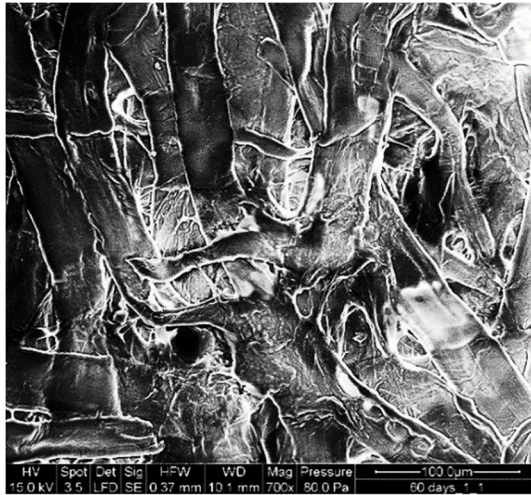
Figure 3.22 SEM image of a 60-days aged pressboard
