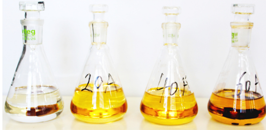
Figure 4.5 Oil colors of aged oil-pressboard samples
