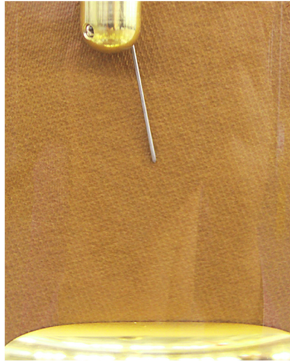
Figure 4.3 The actual arrangement of the needle-to-plate electrode at the interface
