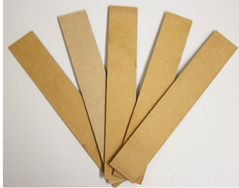
Figure 4.1 Pressboard samples for capillary water rise tests
