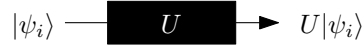
Figure 2.39.: The learning objective is to reproduce whatever the black box does—unitary evolution with U .
