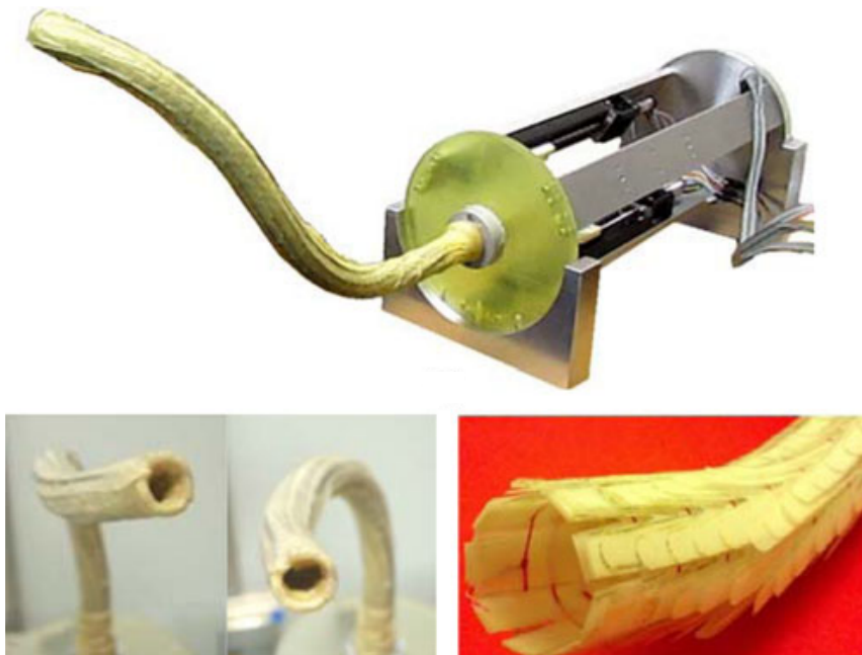
Figure 32: Layer jamming manipulator with helically wrapped flaps and two actuated segments (reprinted from (Y. J. Kim et al., 2013), ©2013 IEEE).
