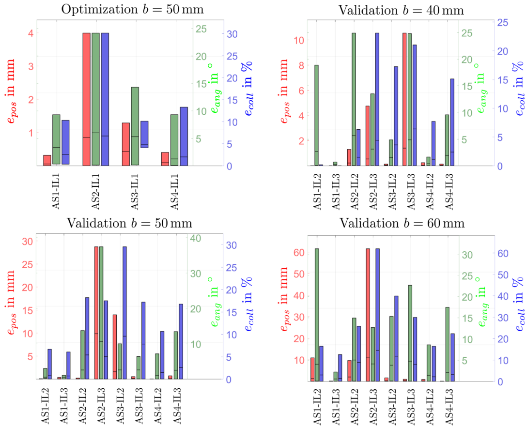
Figure 54: Results of the two segment design third optimization run and validation, showing all three objective errors as box plots for different distances to target points. Errors e_{\text{ang}} and e_{\text{coll}} are converted to degrees and percent for better representation.
