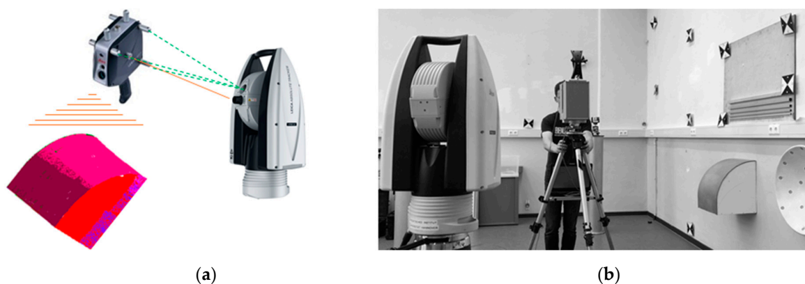
Figure 15. Measurement of the reference geometries at the 3D laboratory of the GIH using T-Scan and laser tracker (a) and k-TLS with laser scanner, laser tracker and T-Probe (b) [22].
