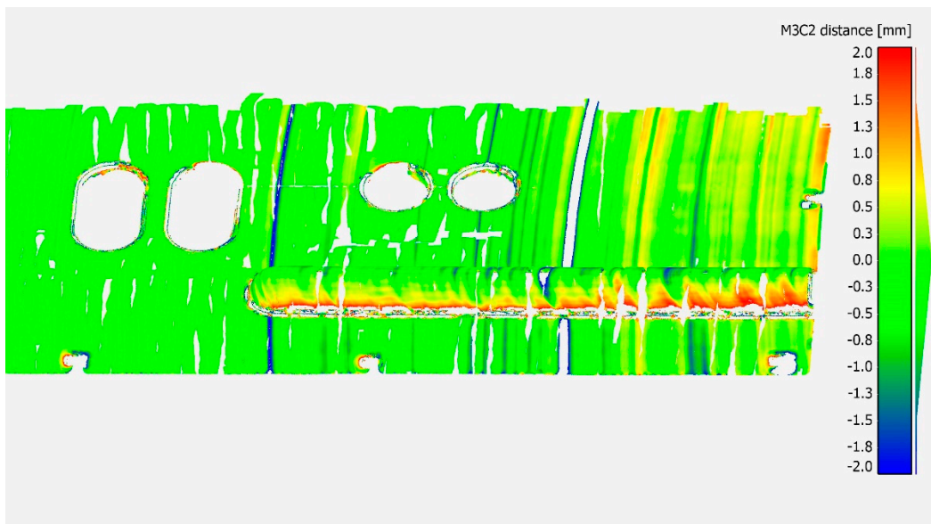
Figure 27. Bottom view on the mock-up showing the M3C2 distances of the 3D point clouds captured with the T-Scan and k-TLS (dolly).
