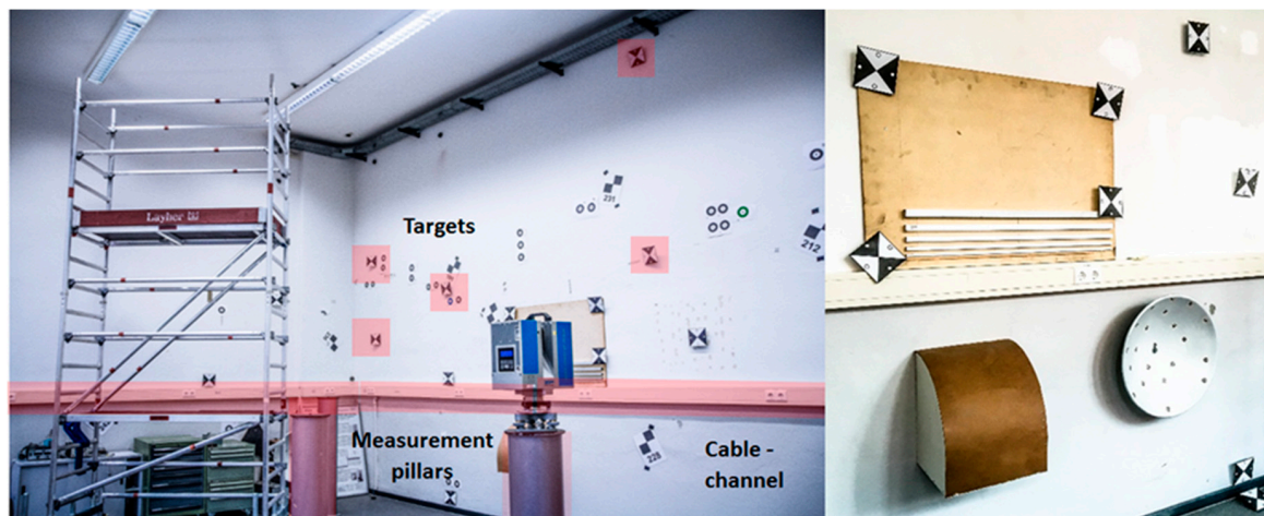
Figure 10. The 3D-laboratory of the GIH with measurement pillars and cable channel (left) and reference geometries (right) [22].
