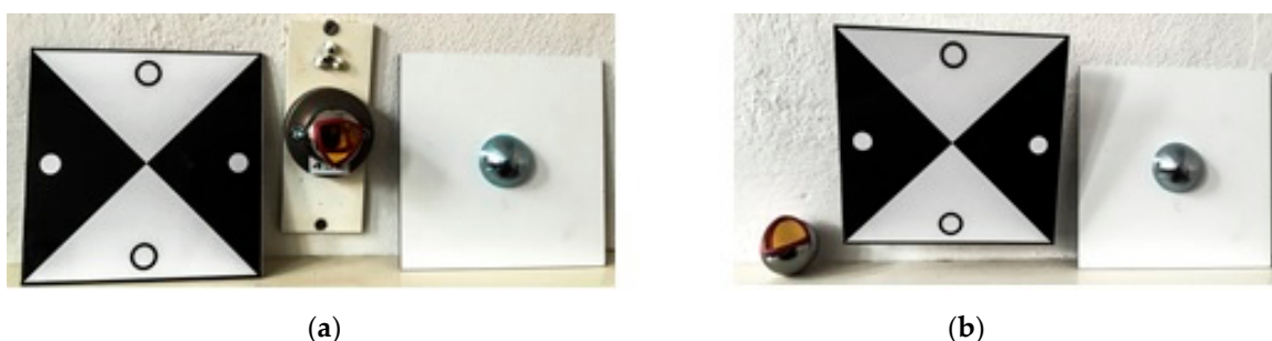
Figure 3. Target mount for the combined adaption of the targets and corner cube reflectors (CCRs) (a) target front, target mount with CCR, target back; (b) CCR, target mount with target, target back [22].
