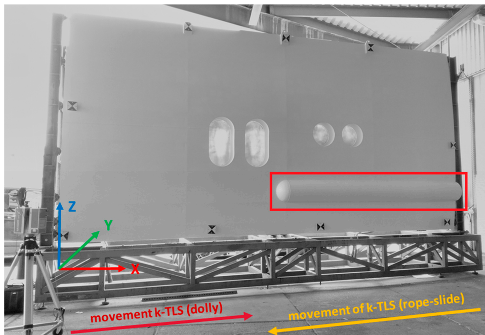
Figure 11. Mock-up with reference points signaled by checkerboard targets (Figure 3), origin of the reference frame. Moving direction of k-TLS and investigated (Section 5) cylindrical geometry marked with red frame.
