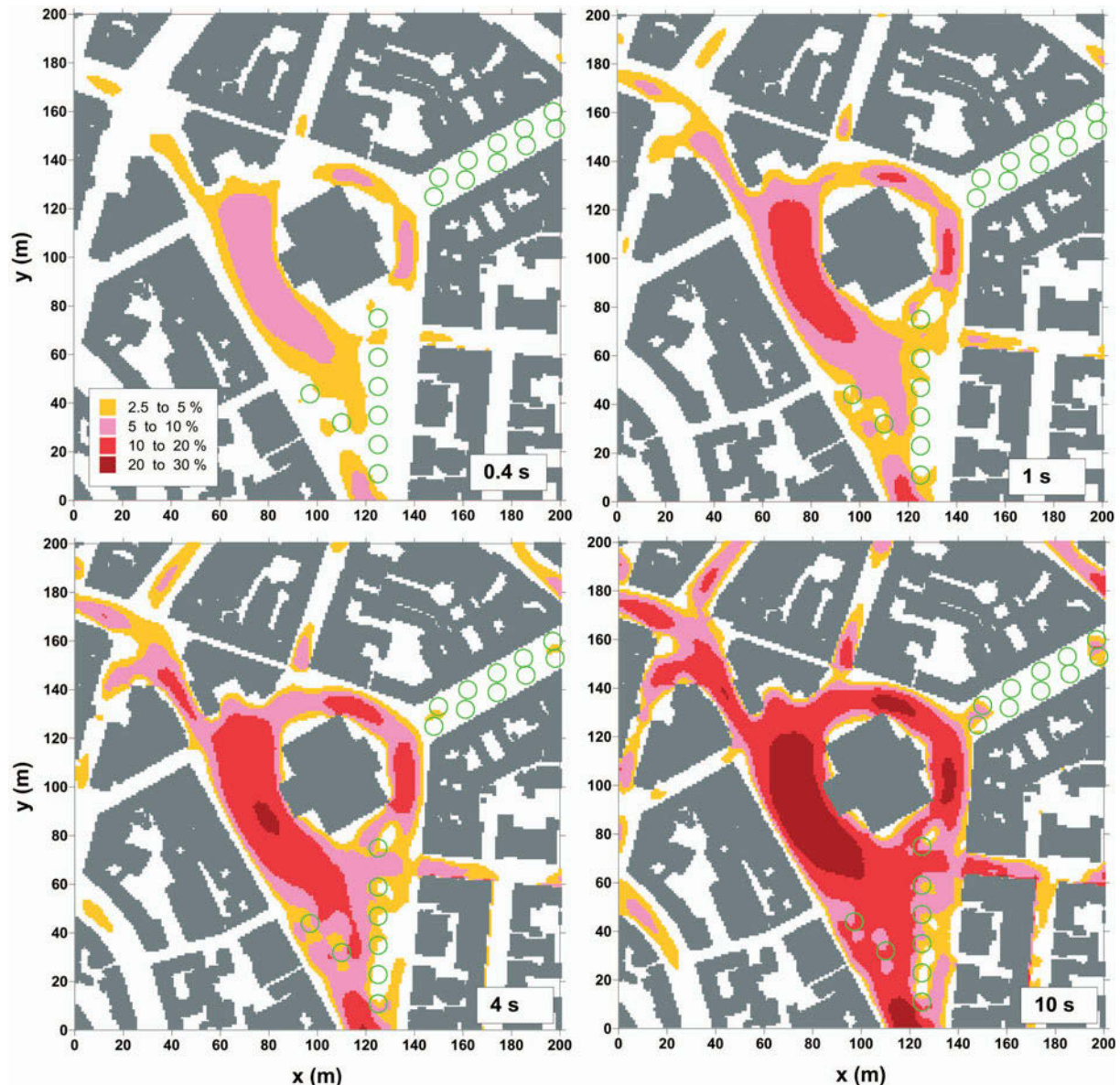
Figure 9: Horizontal distribution of exceedance probability for hours with wind speeds greater than 5 \text{ ms}^{-1} for different gust definition times of 0.4 s, 1 s, 4 s and 10 s.
