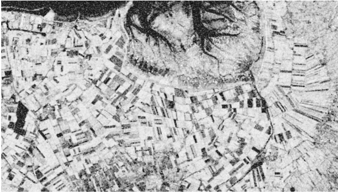
Figure 2-8: Example of a coherence image (Groningen, the Netherlands). Bright parts show a high level of coherence, whereas dark areas indicate a loss of coherence. The loss of coherence in the agricultural fields is mainly caused by temporal decorrelation as the two data sets are acquired in August which is the harvest time in an agricultural area such as Groningen.
