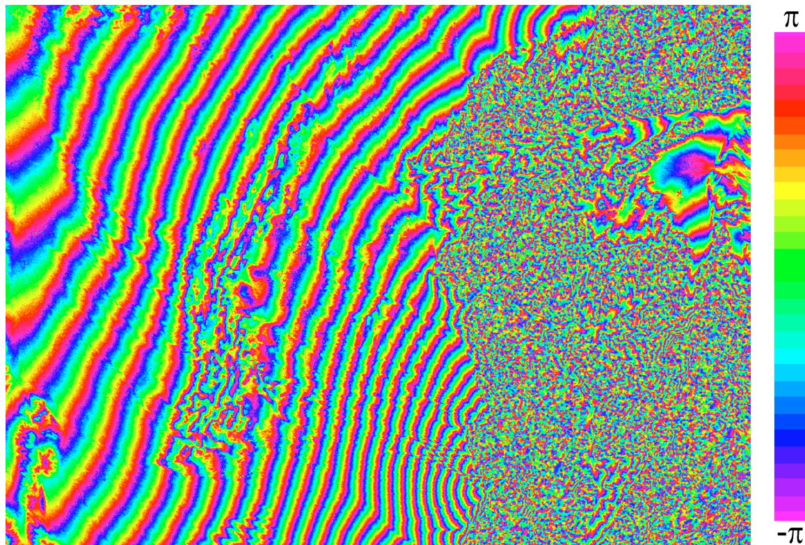
Figure 2-7: Example of an interferogram (Ningxia, China). The interferogram contains the phase difference of the two complex images which is encoded in colour. A full colour cycle represents a phase cycle, also called fringe, covering the range between -\pi and \pi . The number of fringes of a certain distance determines the fringe rate which can be used for the flat earth removal.
