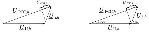
Figure 3. Illustration of the “difference” and “projection” indices
