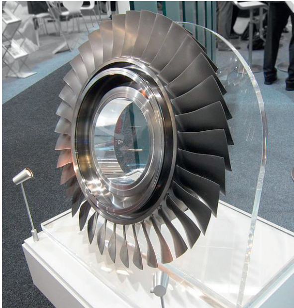
Fig. 1. A compressor blisk on display at the Paris Air Show 2013. This is a single-piece item, generated with 3D CNC milling. Source: Olivier Cleynen
