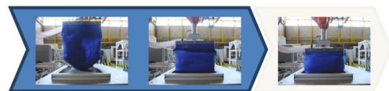
Fig. 9: Test scenario of FormHand with sensor integration. Left: Cushion in soft state, right: the cushion is compacted to a maximum (hard state).
