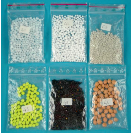
Fig. 6: Selection of granulates (G1 to G6), from top left: EPP, EPS, expanded glass, ABS, rape seeds, cherry pits. See also [8].
