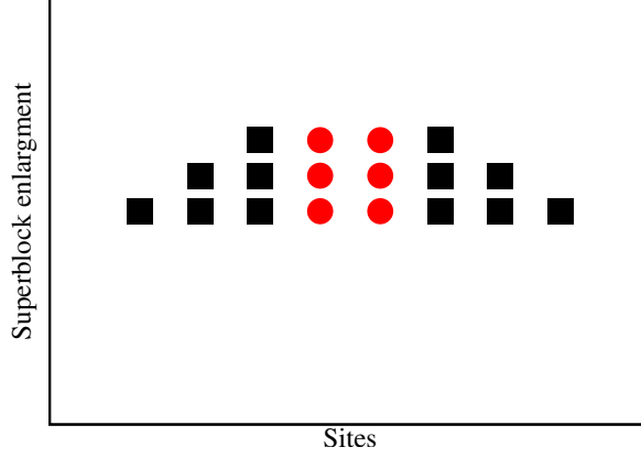
Figure 1.2: Schematic representation of the infinite-system algorithm of the DMRG method. The black squares represent the enlarged system and environment blocks while the red circles represent the added sites.
