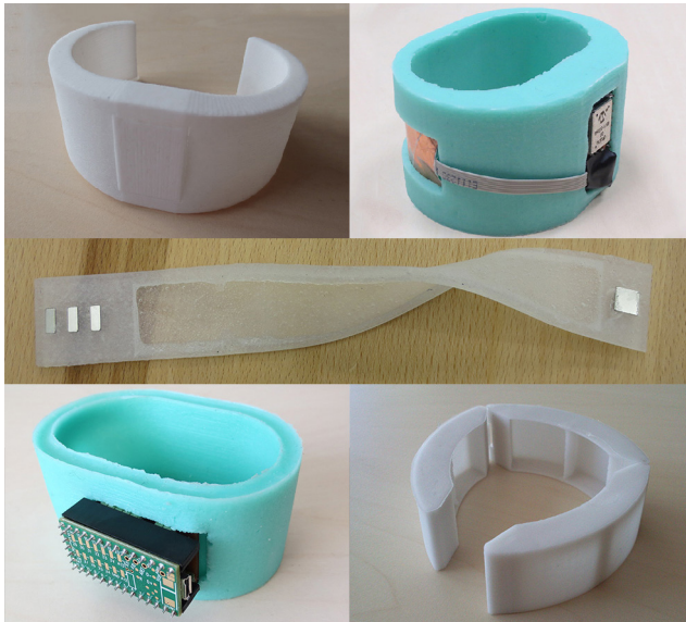
Figure 4.15: Bracelet prototypes clockwise from top-left: (1) 3D-printed rigid open bracelet, (2) final silicone-cast bracelet with embedded electronics, (3) silicone-cast strap with magnetic clasp, (4) 3D-printed segmented bracelet, and (5) first closed silicone cast with electronics.
