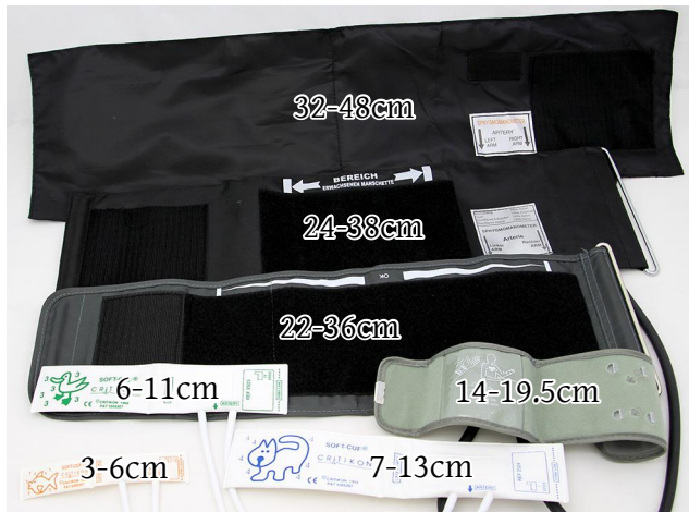
Figure 9.2: We used a wide range of blood pressure cuff sizes to test our system on several body locations. The smaller cuffs can be wrapped around single or multiple fingers, the 14-19.5 cm cuff fits comfortably around a wrist, while the larger cuffs fit around upper arms and legs.
