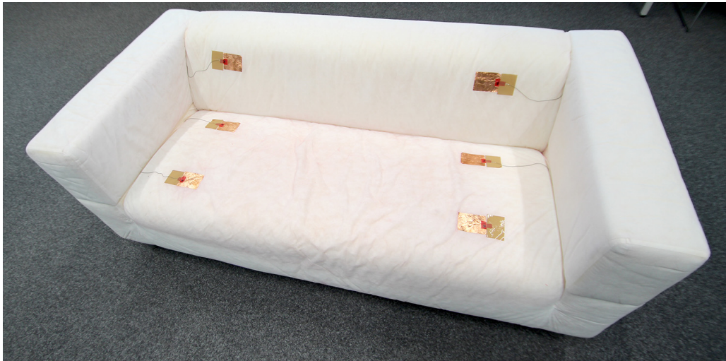
Figure 4.9: We attached six electrodes on the couch, normally hidden underneath the couch cover. Capacitive sensing is still possible through the fabric.
