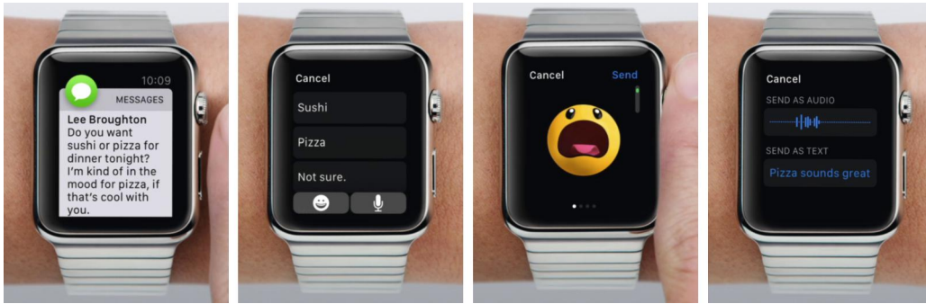
Figure 6.3: The Apple Watch offers different ways to reply to a message. Based on the received message, it generates a set of canned replies that can be send with only one tap. If the predetermined choices are not to a user’s liking, she can also send an emoticon, or dictate a response and send this as either a voice recording or transcript. Dictating the response takes more effort than selecting from canned responses, but also allows more control over the response. All images © Apple Inc.
