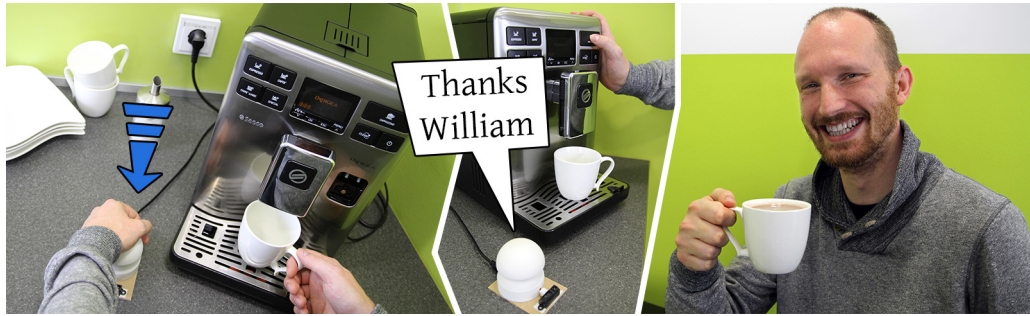
Figure 4.1: Pushing the button next to the coffee machine, William is recognized and his coffee tally is updated. No extra interaction is needed to inform the system who is pressing the button. Recognition and action are integrated.
