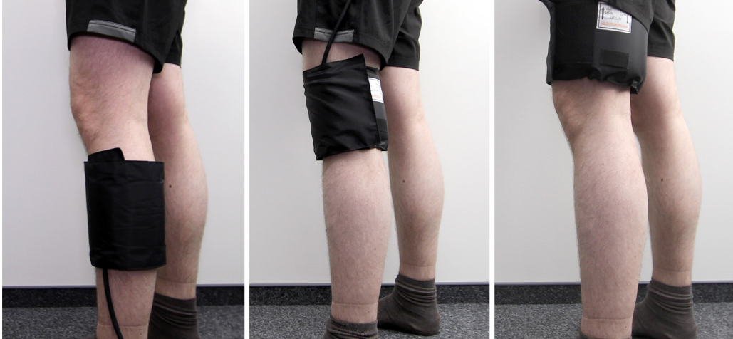
Figure 9.17: Different strap positions enable different sensations on strong inflation. While lower and upper leg placement give a feeling of weighing one down , placement on the knee can effectively lock the leg. Thus one just feels restricting while the other one is inhibiting movement. Straps could be affixed at positions by sewing them into pants.
