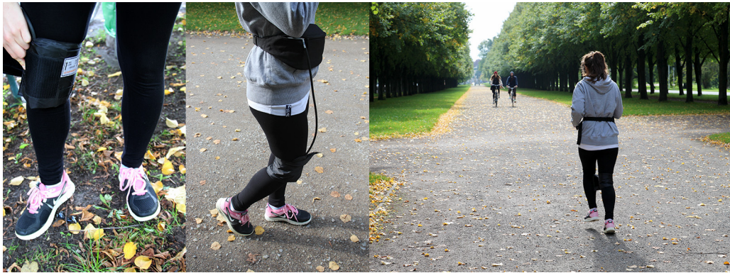
Figure 9.18: We created a jogging game where runners are pushed to reach checkpoints in a given time via compression feedback. Runners wear a compression feedback strap around one knee. The strap is controlled from a controller board in a waist bag.
