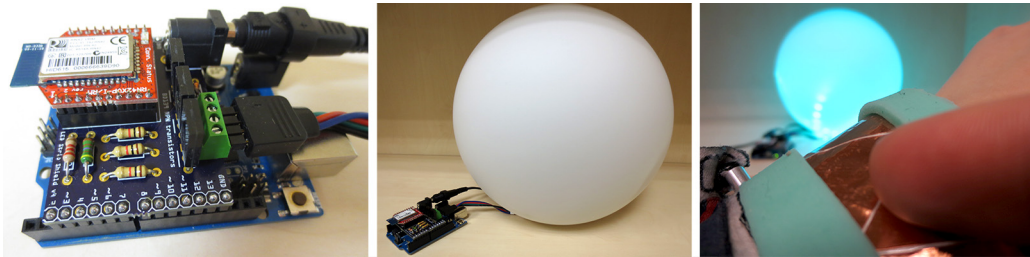
Figure 4.18: Our prototype light setup uses a custom Arduino shield to drive an RGB LED strip inside a spherical lamp. The Arduino receives commands over Bluetooth and updates the LEDs' color accordingly.
