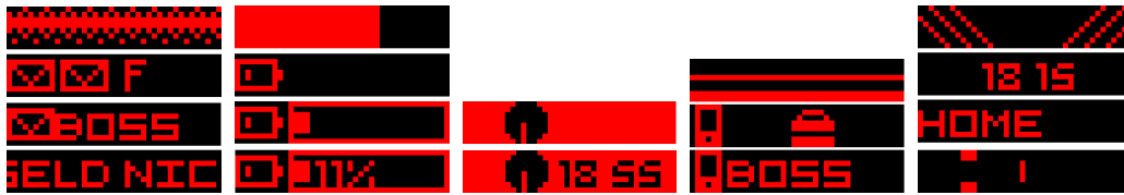
Figure 3.13: Display design for different notifications: messages, battery, clock, calls, alarm. Each row shows a different distance-dependent state with coarse feedback at the top. Thus, the lower the row, the more granular the feedback. For example, the messages first show just a message indicator animation, then an icon for each available message, then who a message is from, and finally the message subject.
