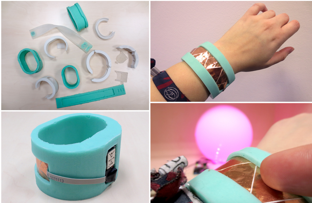
Figure 4.12: Our light-control bracelet is made out of silicone, has an embedded micro-controller, and can sense touch and gestures. It allows changing the hue and intensity of a light at three different levels of control.
