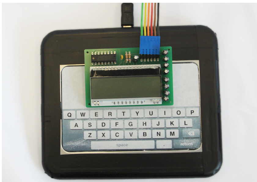
Figure 5.3: We modified a Synaptics ForcePad to allow for graphical feedback to users while typing by attaching an LCD display on top of the device. The display is controlled via an Arduino (not shown). A modified version of the iOS landscape keyboard is glued to the device. Shift, voice-recognition, and mode switch buttons were removed and the space key extended to encompass the @-key.
