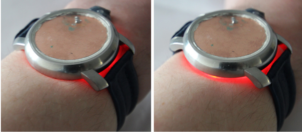
Figure 8.4: When wearing the watch directly on the arm (left) it sits tighter than when using the silicone padding (right). The slight gap due to the silicone also leads to additional light on top of the scattered one.
