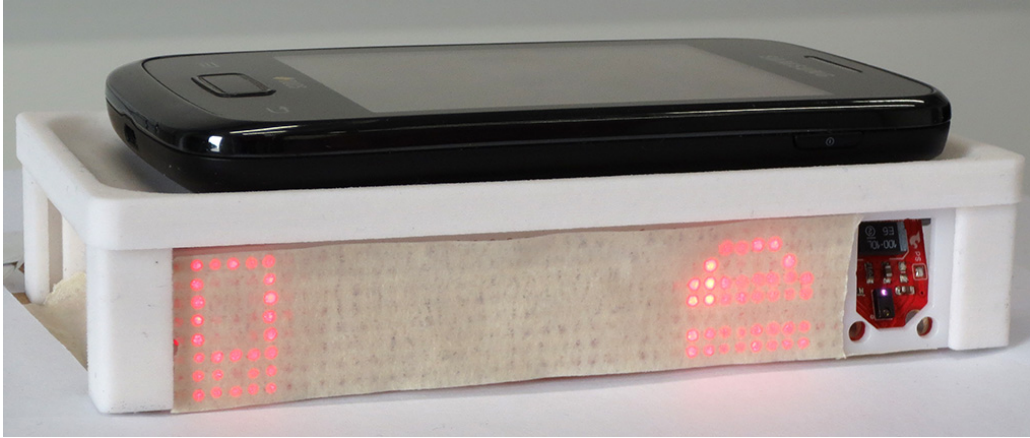
Figure 3.9: Our prototype emulates future phones with high brightness displays at their side. It consists of a red dot-matrix LED display and a proximity sensor mounted underneath a phone.
