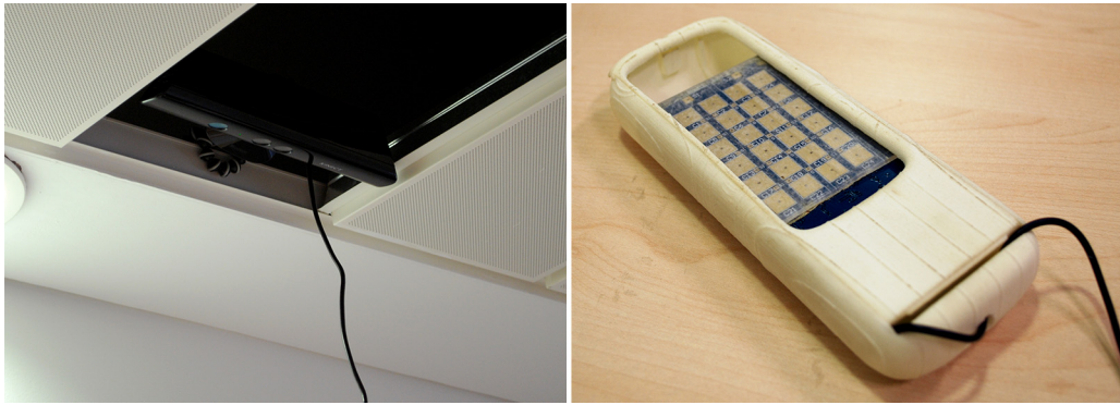
Figure 2.3: Ceiling mounted Kinect (left) and SHAKE SK7-ExtCS1 capacitive sensing extension board (right) used for the study prototype. This setup allowed for the necessary on and above the device sensing.
