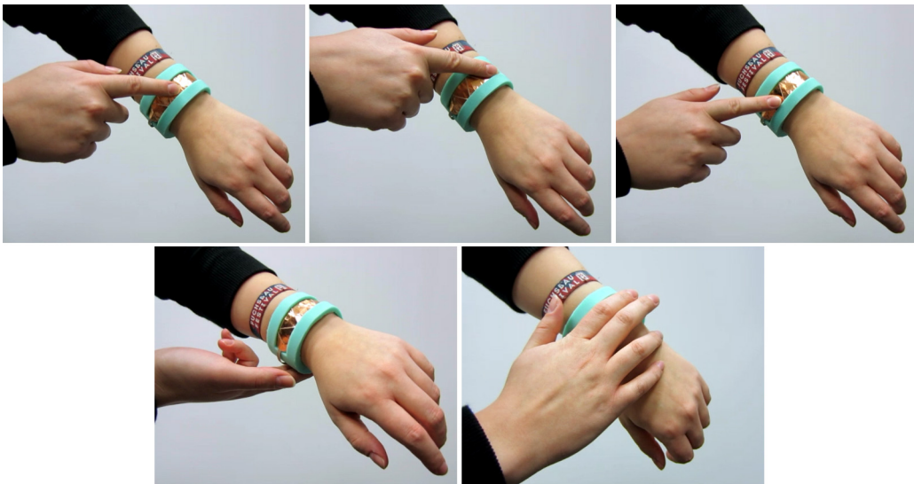
Figure 4.19: We distinguish several different touch gestures (from left to right, top to bottom): (1) moving along the slider, (2) touching the leftmost segments of the slider, (3) touching the rightmost segments of the slider, (4) tapping on the device embedded in the back of the bracelet, and (5) covering the whole slider with a hand.
