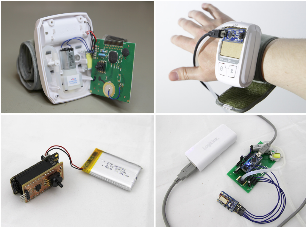
Figure 9.3: We built several compression feedback controller prototypes. They all reuse parts from off-the-shelf blood pressure monitors (shown in upper left image). We only keep the sensor and valves at the wrist for our first prototype (upper right), but move the pump to reduce its influence on the sensation. The second prototype (lower right) is designed for mobile evaluation, fits into a pouch, and is controlled from a phone via a Bluetooth module. The third prototype (lower left) miniaturizes this setup for even better mobility.
