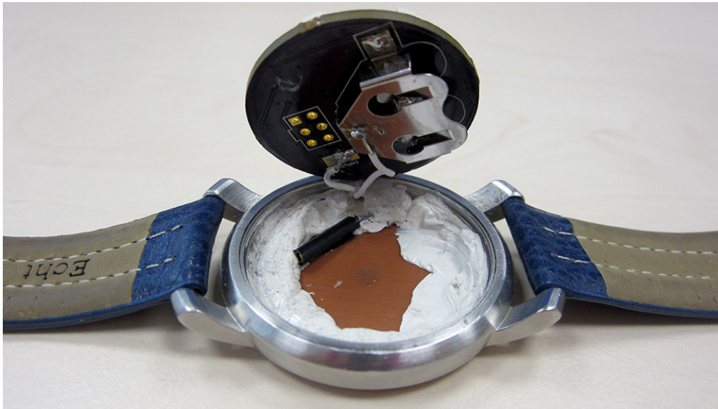
Figure 8.5: The bottom of the PCB holds a coin cell battery with enough power to run the prototype for a day. We sealed the front of the watch to prevent light leakage to the front. The used putty also holds the PCB in place and prevents damage due to free movement inside the case.
