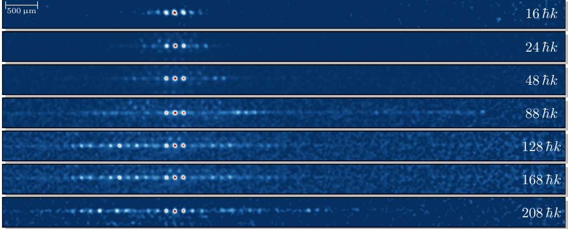
Figure 7.8: Exemplary density plots of closed interferometer output ports. The losses due to the initial double Bragg diffraction are visible in all cases almost equally around the output ports, but significantly increased losses can be observed for the lattice acceleration with separations of \geq 88 \hbar k .
