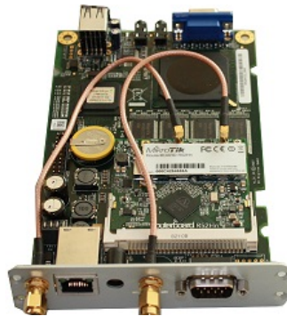
Figure 18: A detailed view of the embedded PC and the wireless radio board.
