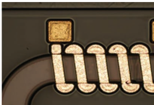
Figure 3. Deposited top layer of the copper
