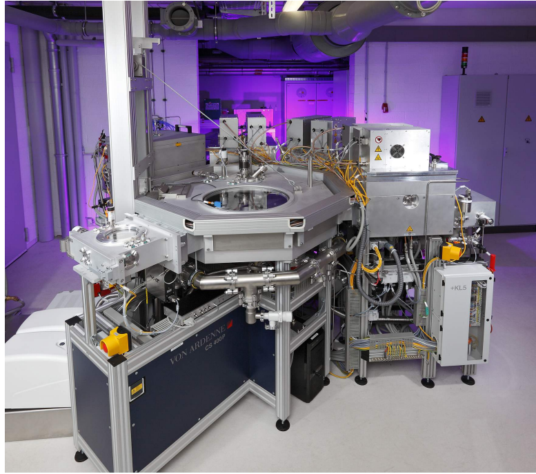
Figure 3.1: Photograph of the PECVD Cluster System CS 400 P (von Ardenne, Germany) used in this study.
