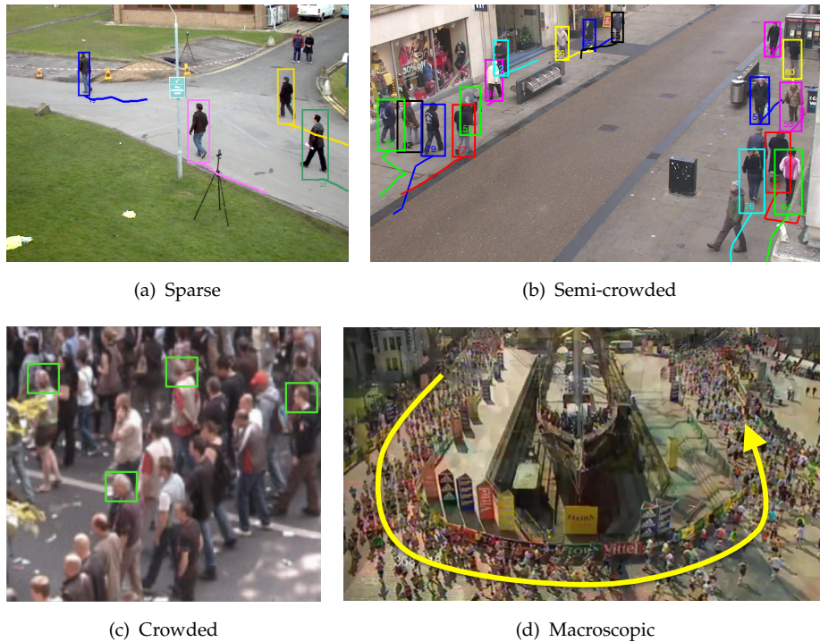
FIGURE 2.1: Scenarios with different crowdness levels. (a) Sparse: individuals are detected and tracked throughout the scene. (b) Semi-crowded: it is still possible to detect individuals, but occlusions and missed detections are very common, making tracking challenging. (c) Crowded: tracking full-body pedestrians is no longer possible, but detection and tracking of heads is still performed. Person counting is a common task for videos of this crowdness level. Image from [22]. (d) Macroscopic scenario: individuals cannot be properly detected, therefore the goal in these scenarios is typically to find the overall flow of the crowd. Image from [25].
