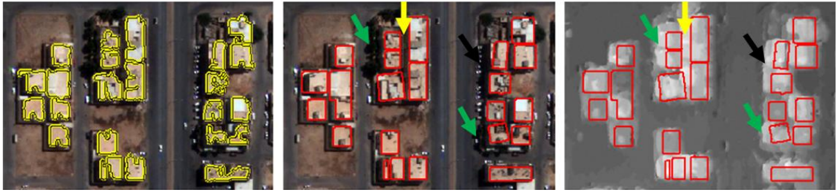
Figure 49- Delineation of building footprints using 3D segmentation (left): segmentation of building rooftops, (centre): building outlines superimposed to original image, (right): building outlines superimposed to DSM derived from SGM
