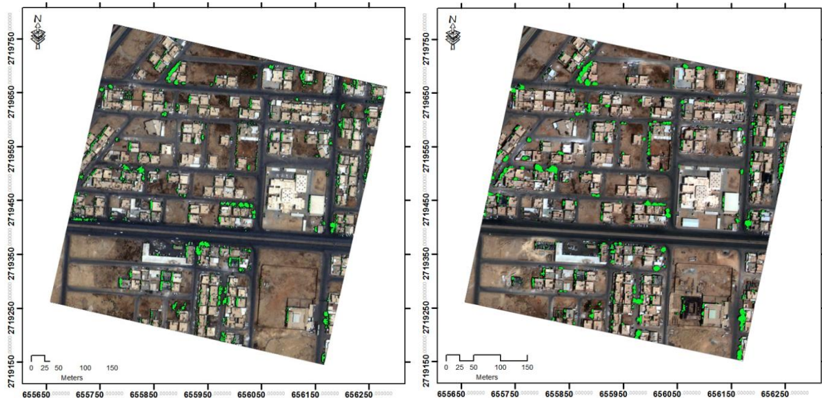
Figure 38- Vegetation mask derived from MLC classification using (left) IKONOS image, (right) GeoEye-1 image
