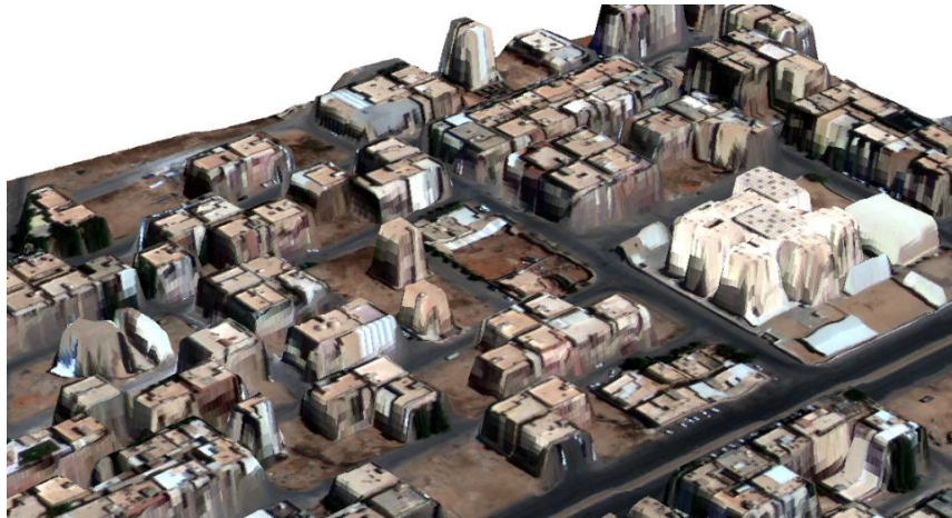
Figure 44- Building 3D visualization based on the DSM enhanced with GIS polygons
