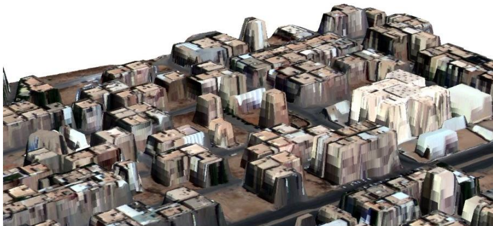
Figure 53- Buildings 3D visualization using final enhanced DSM
