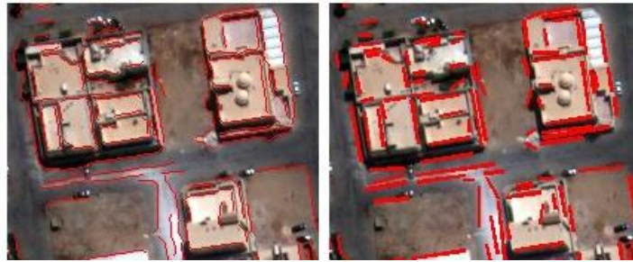
Figure 45- Straight line detection: (left) edge detection using the Canny algorithm and then finding straight edges by a PCA-based method; (right) fitting a straight lines on edges based on the Douglas-Peucker line simplification
