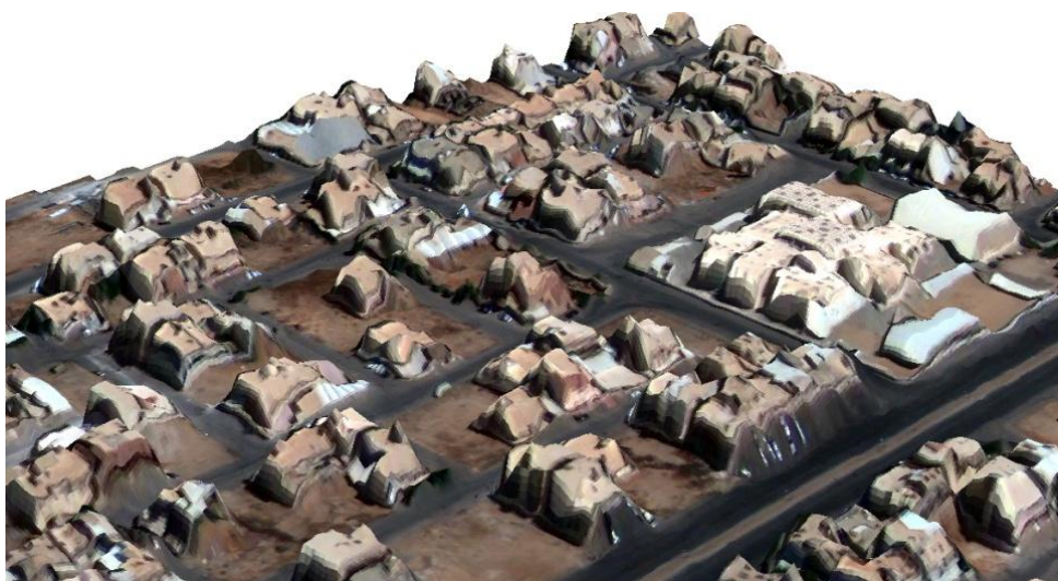
Figure 41- Buildings 3D visualization based on the DSM derived from SGM
