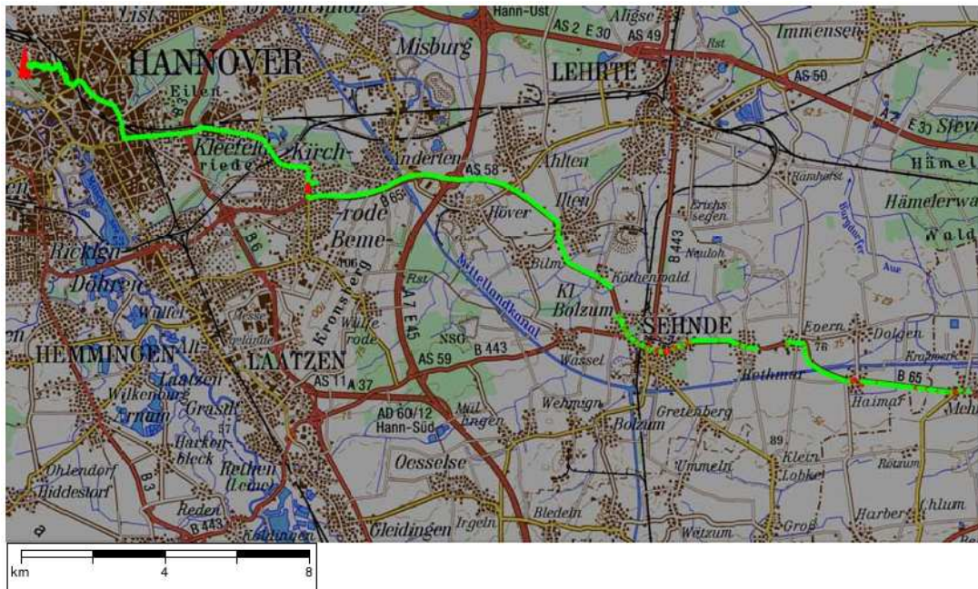
Figure 4.7: Field strength measurement of the coverage limit, 4 QAM mode (code rate: 0.33), start of the measurement at the transmitter on the left side of the map, stop at right border (map source: Bundesamt für Kartographie und Geodäsie)
