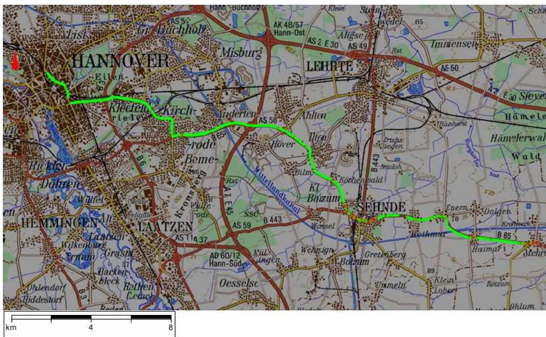
Figure 5.13: Measurement of the coverage limit in 4 QAM mode (code rate: 0.5) in the VHF Band III (green: audio frames ok, red: one or more audio frames corrupted (map source: Bundesamt für Kartographie und Geodäsie)
