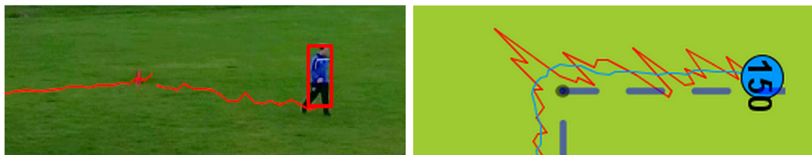
Figure 4. Inaccuracies in trajectories due to erroneous bounding box detections. (Left) The calculated bounding box does not match the object exactly. (Right) The resulting raw trajectory (red line) is afflicted with significant inaccuracies, which are reduced after having applied a filtering technique (blue line).
