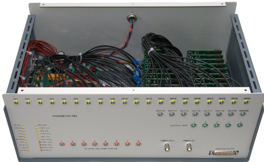
Figure 2.11: LTP-style phasemeter PM3 with 20 input channels. Additionally the transimpedance signals from channel 13 to 20 can be monitored directly with an oscilloscope. The sum of four channels in a row, starting at channel 1, can be monitored, too. Outputs for the bias voltage are also available. The cables of the inputs are shielded.
