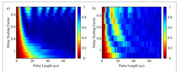
Figure 4. Transfer efficiency for different delay scaling factors and pulse lengths for carrier transitions. (a) Simulation and (b) experimental results of the STIRAP transfer, where 0 (dark red) corresponds to no and 1 (dark blue) to complete transfer. For the simulations and the measurements the ion was initialized in the ground state of motion in  $|1\rangle$  and the pulse length was scanned for different delay scaling factors s.
