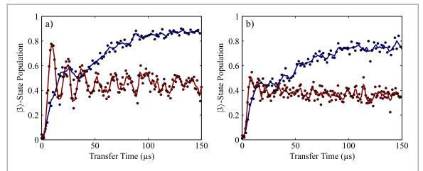
**Figure 9.** Population transfer dynamics of Rabi (red) and STIRAP (blue) for a thermal motional state. The transfer efficiency is displayed for (a) the blue sideband and (b) the carrier transition with the ion initialized by Doppler cooling. The delay scaling factor was chosen to be s=0.5 for sideband transitions and s=0.7 for carrier transitions. The lines are moving averages of the data and are guides to the eye. For clarity the error bars are omitted.
