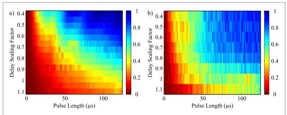
**Figure 5.** Transfer efficiency for different delay scaling factors and pulse length for blue sideband transitions. (a) Simulation and (b) experimental results of the STIRAP transfer, where red corresponds to no and blue to complete transfer. For the simulations and the measurements the ion was initialized in the ground state of motion and the pulse length was scanned for different delay scaling factors s.
