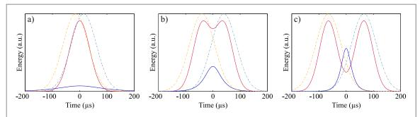
**Figure 2.** Time dependence of the adiabatic criterion. The couplings (left side of (8), blue) and the energy splitting (right side of (8), red) are shown for a fixed pulse length of 100  $\mu$ s and (a) a delay time of 30  $\mu$ s, (b) a delay time of 80  $\mu$ s and (c) a delay time of 130  $\mu$ s. The dotted lines represent the pulses.
