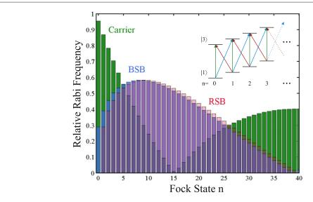
**Figure 7.** Relative Rabi frequencies of the transitions for different motional states of a single  $^{25}$ Mg $^+$ ion in the trap. The values were calculated assuming a Lamb–Dicke factor of  $\eta=0.3$ , corresponding to a secular frequency of 2.22 MHz; green: carrier, blue: blue sideband, red: red sideband. The inset indicates the motional level structure with the corresponding transitions.
