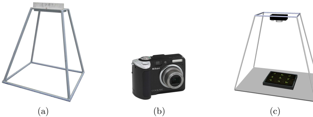
Figure 4.7: Image acquisition. (a) Stand for the camera. (b) Nikon Coolpix camera. (c) Image showing how the pictures of the plants were taken.
