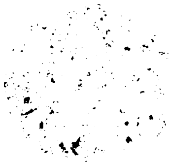
Figure 5.16: Tomogram layer after Gaussian filter and gray scale threshold. The dark areas represent parts of pore structures.
