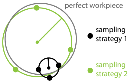
Figure B.3: A perfect circle is measured with two different probing strategies assuming an imperfect CMM with a point coordinate error. In both cases the modelled geometry is not identical to the real workpiece. Again, the first probing strategy yields a significantly larger measurement uncertainty.
