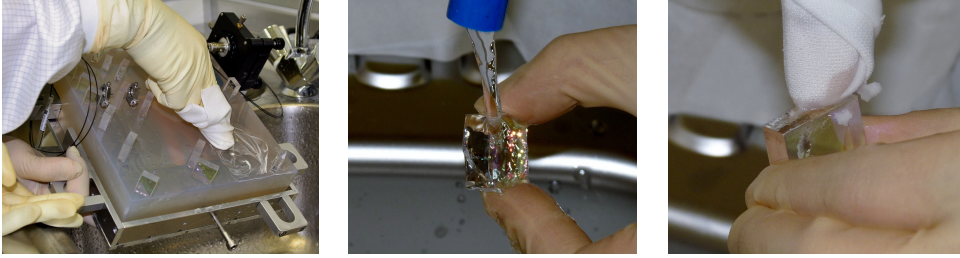
Figure 4.28.: Several cleaning steps during the bonding process: Left: describes the cleaning of the baseplate; Middle: describes the rinsing of the optical component with deionised water; Right describes the cleaning of an optical component.
