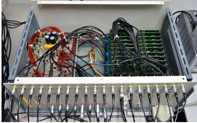
Figure 5.1: Photograph of the hardware-based phase measurement system (PM3) implemented using field-programmable gate arrays with an analogue front-end (20 input channels).
