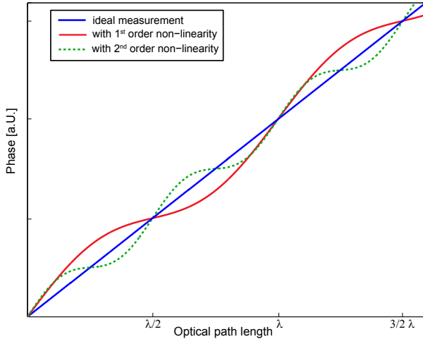
Figure 4.5: Plot of measured phase versus travelled distance. Comparison of an ideal interferometer (blue trace) and one including non-linearity of the first order (red/solid) as well as second order (green/-dashed).
