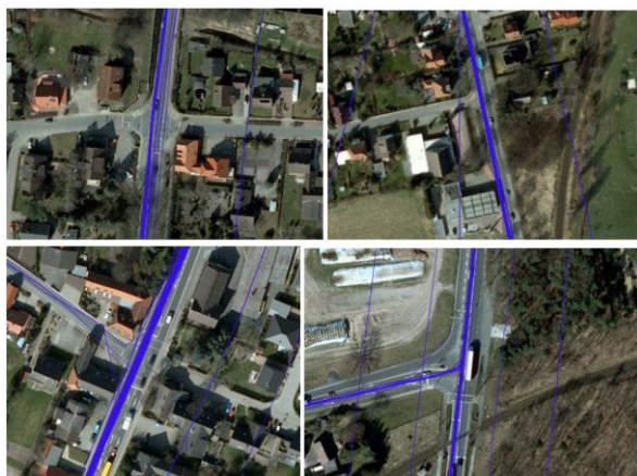
Figure 2. Upper-left: Intersection where no samples (trajectories) exist from all participating road segments that compose the intersection. Upper-right: T-junction where no samples (trajectories) exist from the secondary participating to the junction road. Lower-left: Traffic light-controlled T-junction, where only three samples exist in the dataset that turn
