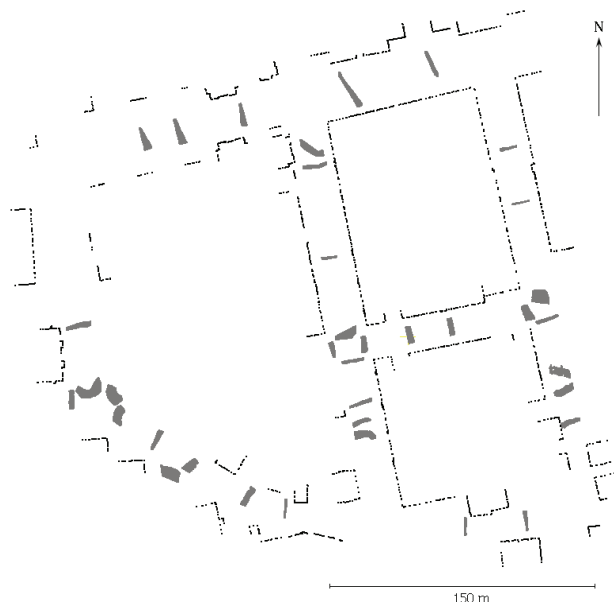
Figure 3. 3D test field with measured points on facades (black) and street profile measurements (gray).
