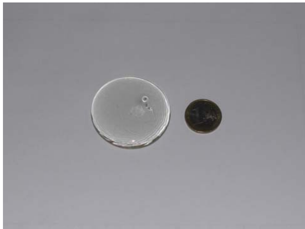
Fig.3.1 An example of a quenched glass (LNKS) in air, quenching was achieved by pouring the molten glass on a brass plate.
