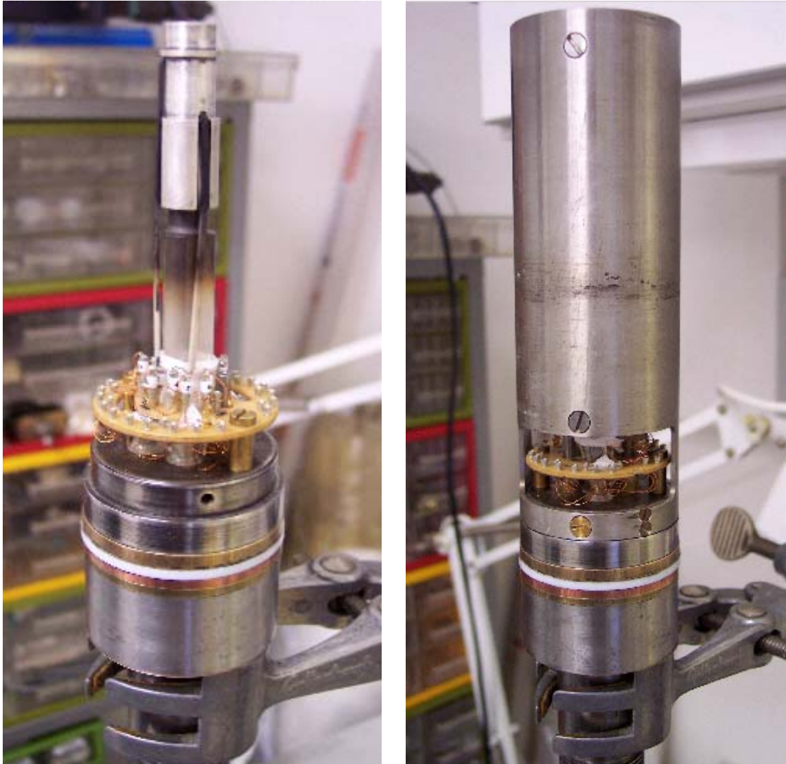
Fig.3.7 On the left side the viscometer sample holder is shown. Sample is within the silver sample tube on top of the silica piston. Thermocouples and glass-epoxy printed circuit board are also visible. On right part is shown the steel cover of the furnace. The inner part of the furnace consists of two heating zones made of Kanthal A1 wires (diameter of 0.6 mm) wound around a tube of sintered alumina (diameter 15 mm) (Schulze et al. 1999).
