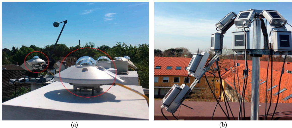
Figure 1. (a) Pyranometers and other instruments available and operational at Institute for Meteorology and Climatology (IMUK); (b) Set of solar sensors based on silicon detectors mounted in several different tilt angles and orientations, operational at the IMUK (IMUK 2017).
