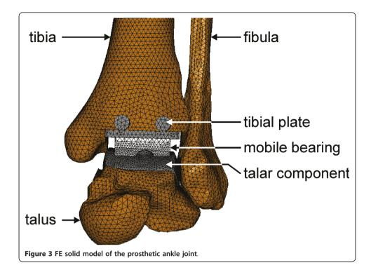
The load was taken from the study of Stauffer et al. [10], in which a load of 5.2 times the body weight had been calculated for the normal ankle joint during the stance phase of gait. A person of 100 kg weight was assumed. Consequently, a static force F of 5,200 N was applied to the tibia and the talus by spreading it equally on ten nodes.
