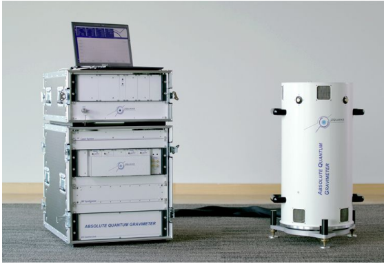
(a) Muquans Absolute Quantum Gravimeter (Muquans, 2017).
