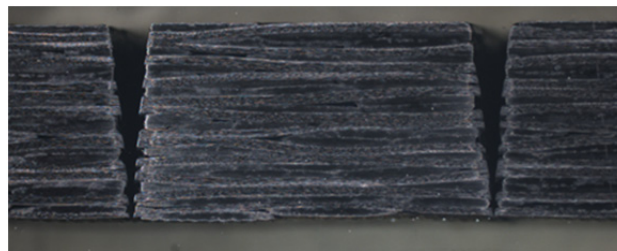
Fig. 6. cross-section of a cut through h = 5 mm material with single-line strategy
