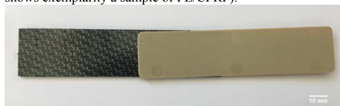
Fig. 5. Laser transmission welded PE/CFRP sample.
