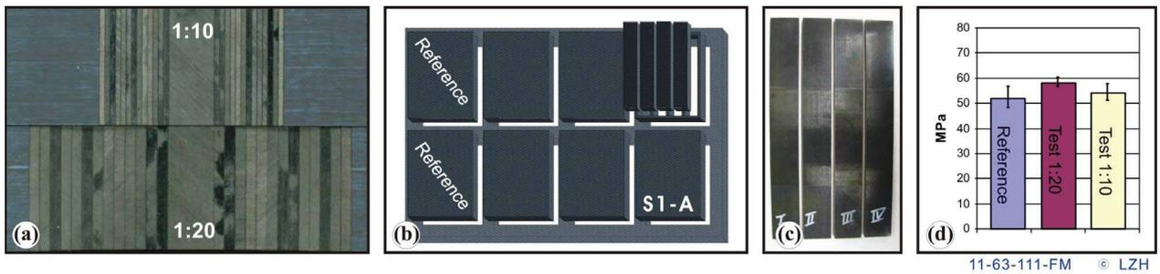
Fig. 6. Bonded repair: (a) size of area with different step width; (b) test pattern according to DIN 65148; (c) separated test specimen; (d) results of shear strength tests in comparison to non-machined specimen (reference).
