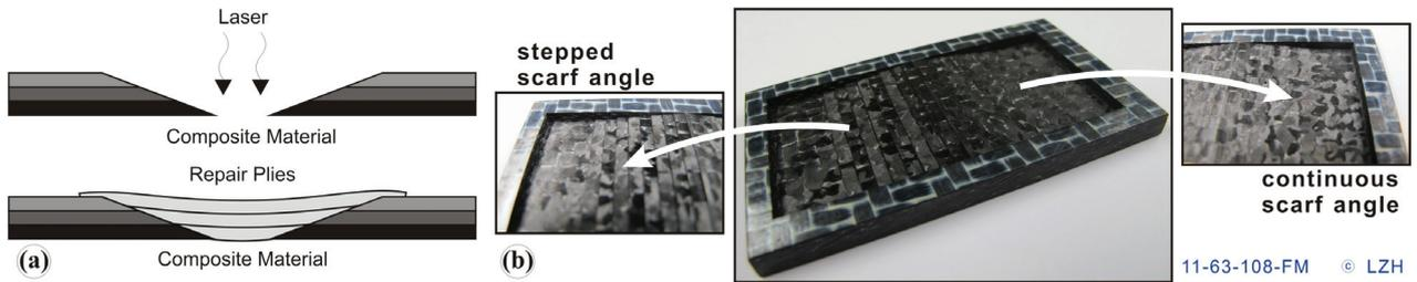
Figure 8. (a) Principle for bonded repair with continuous scarf angle; (b) laser-machined part for demonstration of a continuous scarf angle.
