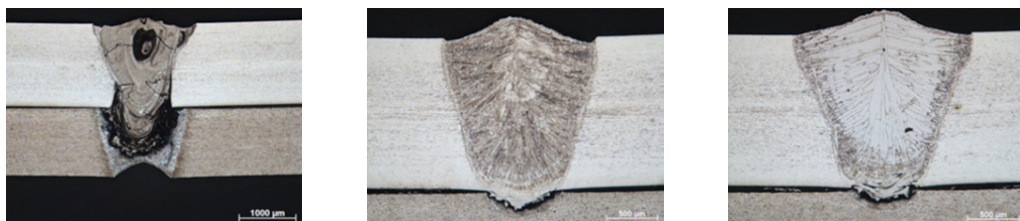
Fig. 9. Cross-sections of laser beam welded dissimilar joints of 1.4301 ( t = 1.50 mm) and AA6016-T4 ( t = 1.15 mm) with a varied energy per unit length of 48.91 kJ/m [left], 46.88 kJ/m [center] and 45.00 kJ/m [right].
