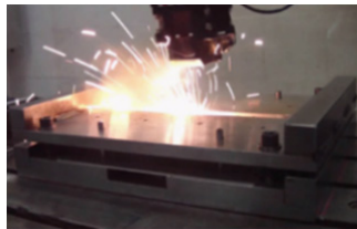
Fig. 4. Laser beam welding of different dissimilar joints of steel and aluminum alloys.
