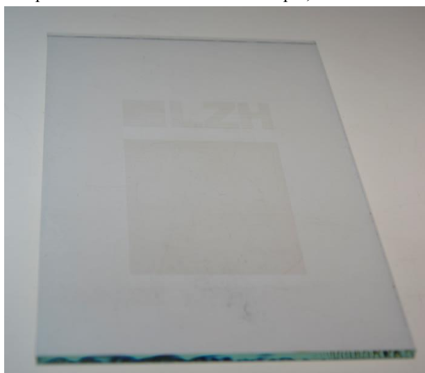
Fig. 7. Selective laser annealed sol-gel coating of \text{TiO}_2
