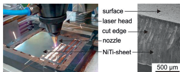
Fig. 4. Pulsed Nd:YAG laser cutting of 1 mm NiTi-SMA sheets (left). Exemplary SEM picture of the cut surface after the cutting process (pulse duration = 1.0 ms, pulse energy = 0.8 J, processing speed v = 3.3 m/s, f = 100 Hz) [6].
