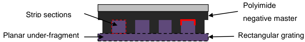
Figure 52: Fabrication model of a rectangular grating with a PI negative mold.
