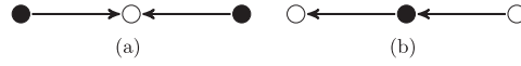
Figure 2. Two different three qudit cluster states. Solid (open) circles represent even (odd) vertices. The simple structure of these graphs means that a vertex ordering is not required to specify the relevant cluster state. (a) An even–odd–even three qudit cluster state. (b) An odd–even–odd three qudit cluster state.
