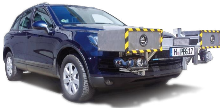
Figure 3. Pixel light system prototype developed at IPeG mounted onto the vehicle used for the experiment.
