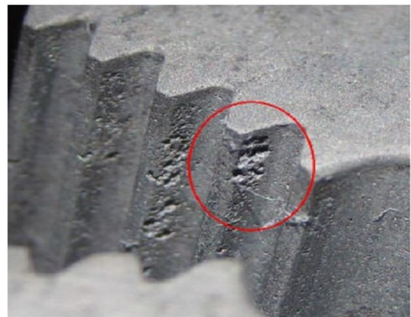
Fig. 1. Corrosion pits at the firtree joint of an HPT disc.
