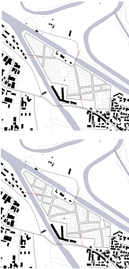
Figure 10.6: (above) Preliminary tests of the block and parcel subdivision algorithm developed by Schneider and Bielik applied to the Limmer Wasserstadt in Hannover.
