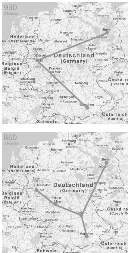
Figure 8.7: (above) Adding nodes (up to a certain point) can make the total network length shorter.
