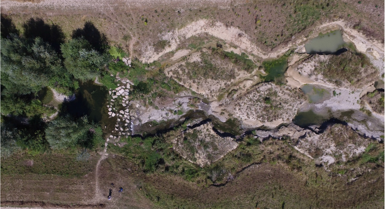
Figure 11.6: (above) Drone based photo of George Descombes L'Aire River Restoration project showing erosion as the water channel finds its own ideal course.
