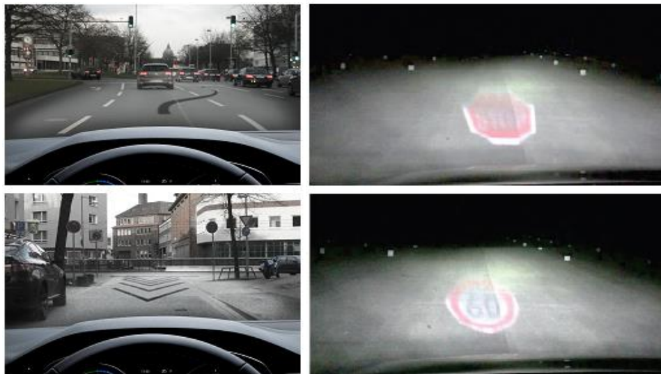
Figure 2. Left: Exemplary functionalities of DMD based automotive lighting units (Renderings) 1 . Right: Scanned working projections from a laser scanning module overlaid on low beam 3 .
