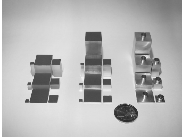
Fig. 2.2. All used test samples with the same graphite coating. Left: B270 cuboid samples. Middle: aluminum cuboid samples. Right: With a cone 'modified' aluminum test samples. All viable apertures are 4x4 mm 2 , 10x10 mm 2 and 20x20 mm 2 . The respective lengths are 2 mm, 8 mm, 20 mm and 40 mm.
