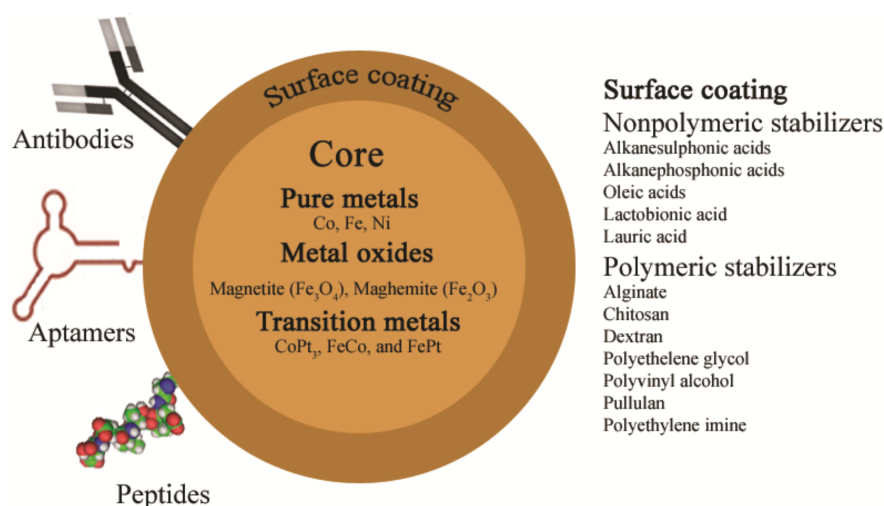
Figure 2. Composition of magnetic beads (MBs) used in analytical applications.
