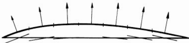
Figure 2.3 Influence of the cambering and the boundary condition: no flow through skeleton line (Melin, 2000).
