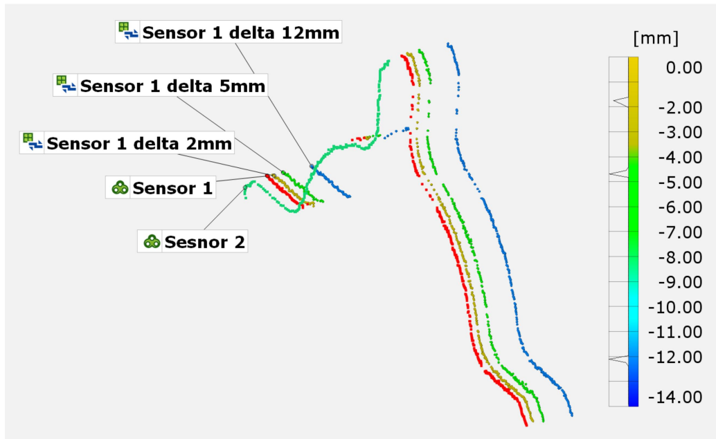
Figure 5: Pure translation of Sensor_1 by 2mm, 5mm, and 12mm. Results of the detected sensor translations and their distributions can be seen in the legend.
