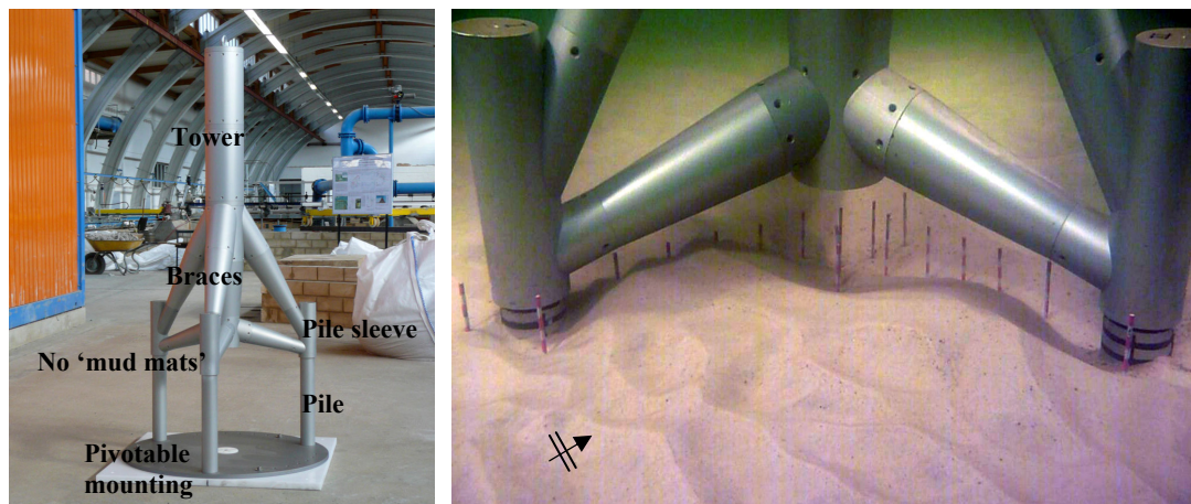
Figure 3. Left: 1:40 Tripod model with pivotable mounting. Right: Typical scour formation in a test series with regular waves after 7000 wave cycles (underwater picture).
